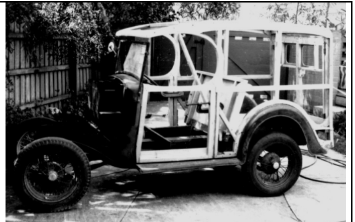
The van under restoration, the body had been destroyed by some photos and one remaining panel helped its rebuild
