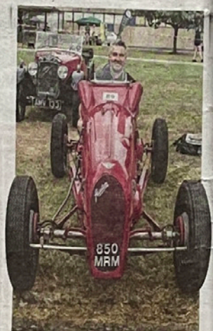
Adam Wragg in one of his father's creations, an Alan Wragg special, 850 MRM, aka Wragg Racer, is one of 12 Wragg 7 Special MkIIIs. Some models were supercharged, some adapted to run on methanol. All were single-seater conversions built on the Austin Seven chassis.
