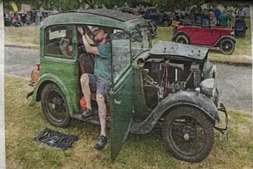
Nick Forrester sets about re-fitting his 1936 Austin Seven ARQ Ruby Mk1's door pillar trim, after replacing the trafficator at the fair once he'd bought a replacement part.
