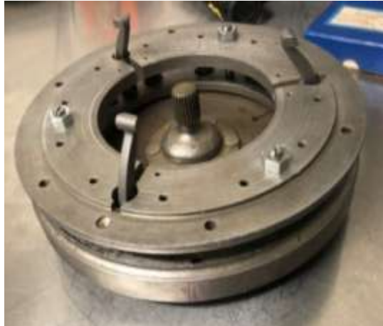
Clutch cleaned up and mated with driven plate and flywheel
