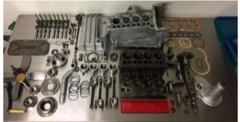
and it took several hours to sort this out. In reality, I only got it to a point I thought was satisfactory but not great. Later that day, I adjusted the camshaft float as I found the new version was not providing sufficient clearance for the oil to depart the brass bush.
