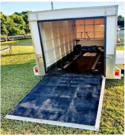
Tandem trailer to suit a short wheelbase Austin 7, internal dimensions 3.9 m. long x 1.8 m. wide by 1.74 m. high, overall length from the tow hitch to the tailgate is 5.32 m. Steel rear door doubles as loading ramp, floor all steel with built in tie points.
